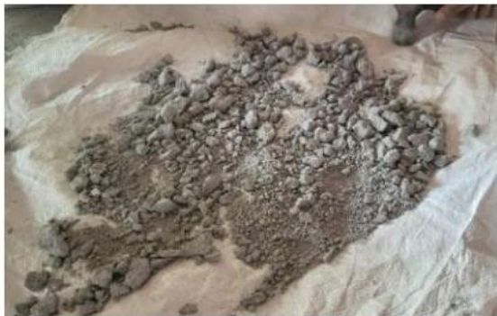
Fig 3 :: AAC Waste being prepared
